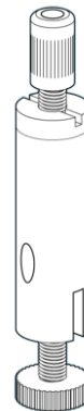
BELT 1084.0502 Griplock Integrated Balancing Cylinder with Safety Lock All Beretta Griplocks are for a maximum load of 15kg to allow a 5:1 safety factor
